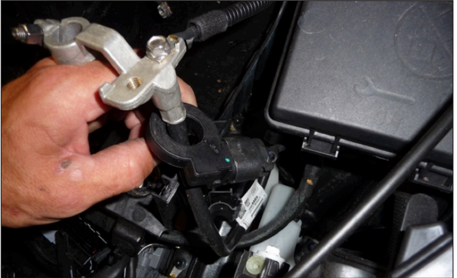
Remove intake hose and throttle body:
