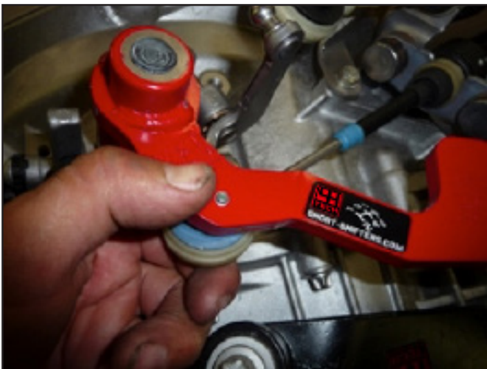
Click the 2 shift cables back on the bolt heads.
