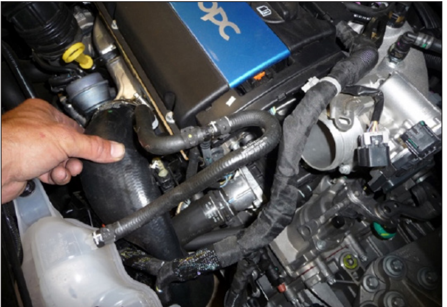
Remove intake hose and throttle body:
